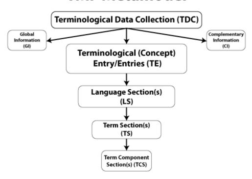
Figure 1. High-level structure of the TMF (ISO 16642) metamodel
